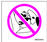
SRS decal at far right of the passenger's dashboard
