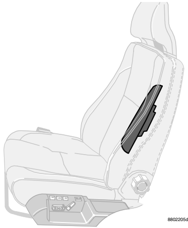
Location of the side impact (SIPS) airbag
