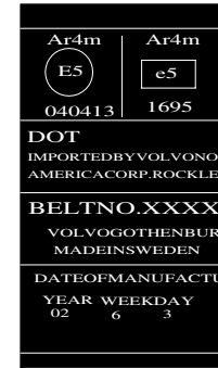
Sample label on all seat belts with tensioners
