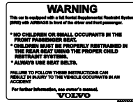
SRS decal at far right of the passenger's dashboard
